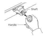
Wind up the handle at clockwise direction to store the ladder.
