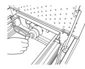
3 Put the handle into the shaft.
