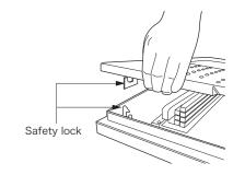
B Lift up the upper lid slightly to confirm the safety lock is locked.
